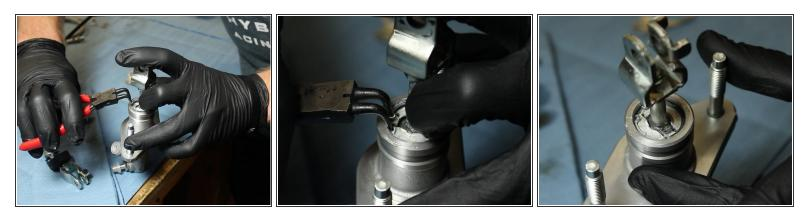
Using the C-clip pliers, insert the OEM rod & fork into the EM1 CMC. The EM1 dust boot is optional.
