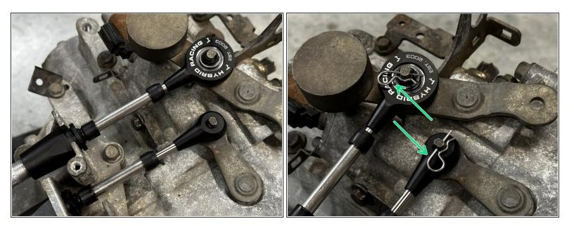
Note the orientation of the shifter cable end link. Make sure the Hybrid Racing logo is facing up and the insert is flat against the gear selector.
