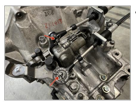
Install the supplied cotter pins in both cable end links.
