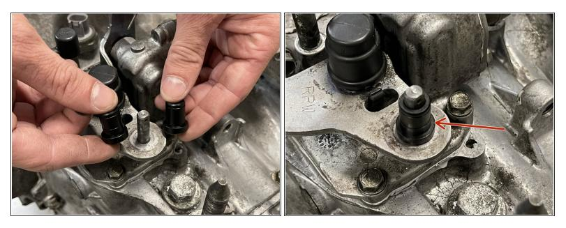
Before you begin, you must select one of the two included spacers. The spacer should fit precisely on the gear selector pin.
