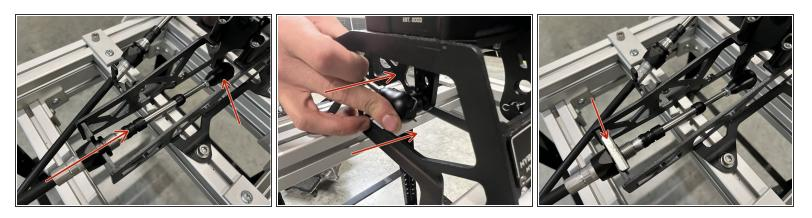
Insert the shifter cables through the shifter base and secure them to the shifter with cotter pins. We
