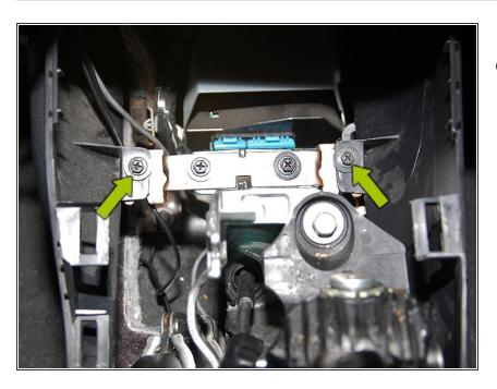
Next you will need to use your 8mm nut driver (Phillips head screwdriver will work) to remove the (4) bolts that hold the center console down. The front (2) are right in front of the shifter.
