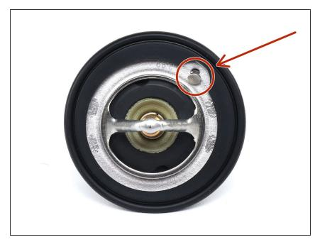
Make sure the pin valve is at the top when installed. Do not install it upside down; otherwise, air will get trapped, and it will not bleed properly.
