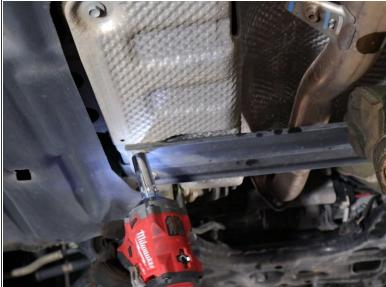
Remove the lower chassis brace.
