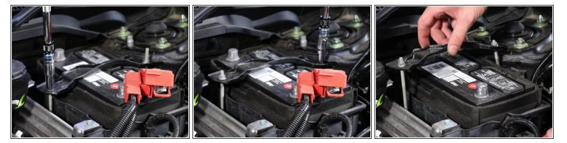
Unbolt and remove the battery tie-down bracket.
