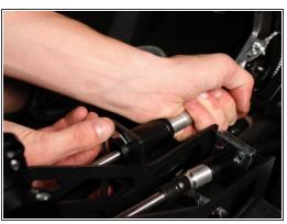
Inside the car, attach the cables to the shifter.
