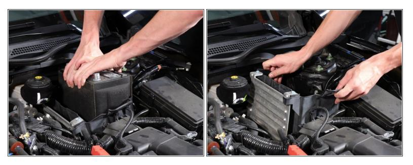
Remove the battery from the car. Then, remove the battery isolator.
