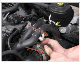
Loosen the air inlet tube and remove it. Be sure to move the hoses out of the way.
