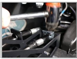
Reinstall the shifter cable clips and secure them in place with a mallet if necessary.
