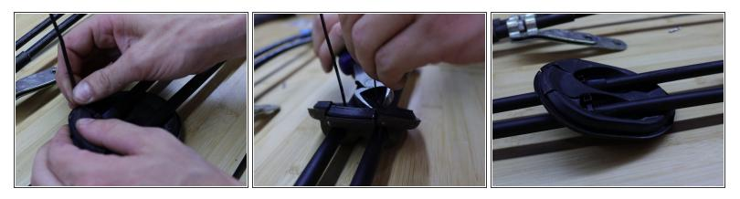
Secure the floor seal with both supplied zip ties. These ties help the cable stay in place.
