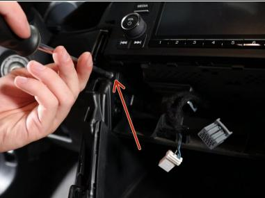
Remove the two phillips screws holding the side console trim sections in place.
