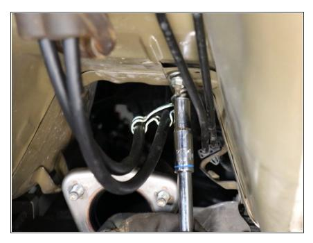
Under the car, slide the cable bracket into place and secure it back into place.
