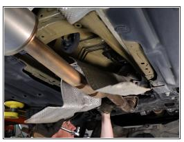
Unbolt and remove the lower heat shield. This will expose the shifter cables.
