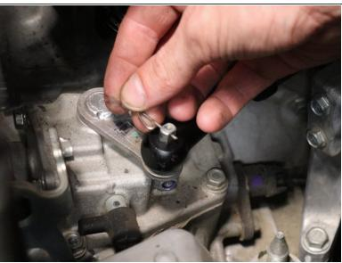
Secure the shifter cable end links with the supplier cotter pins.
