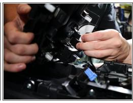
Lift the shift boot cover upwards and unplug all of the electrical connectors.
