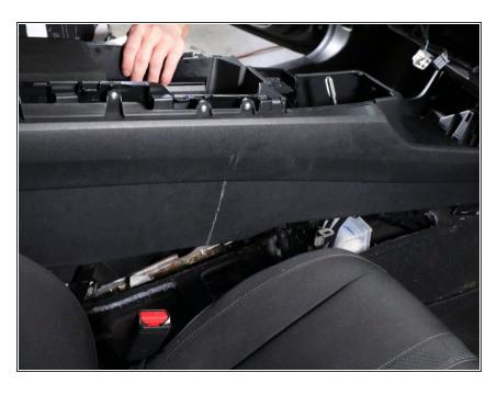
Lift the console up and slide it backward. Remove it from the car.
