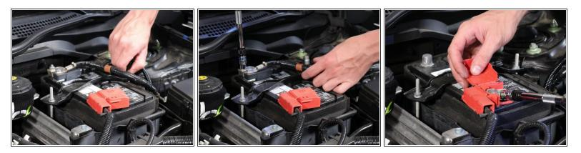
Remove the battery terminals, start with the ground first.
