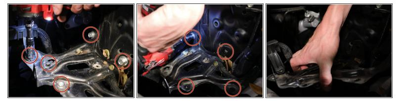
Unbolt the battery tray and remove it from the car.
