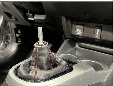
Begin by removing the shift knob and collar if so equipped.
