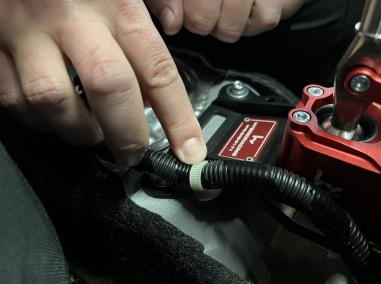
Reinstall the factory wiring harness so it clips into the shifter base.
