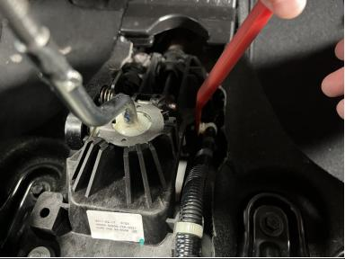
Remove the factory wiring harness from the stock shifter assembly.
