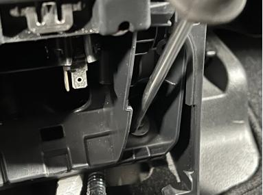
Remove the two rear mounting screws from the base of the console.
