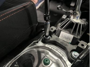
Remove the four shifter base mounting bolts.
