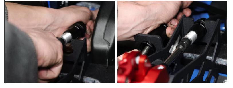
Insert the shifter cables back into the shifter.
