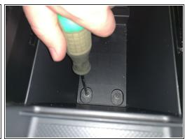
Remove the two screws inside of the center console.
