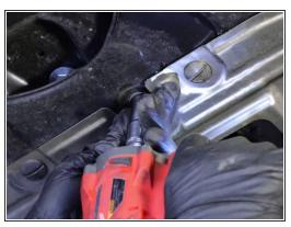
Under the car, remove the plastic under tray to gain access to the heat shielding and exhaust.
