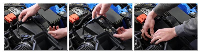
Unclip the MAF wiring harness from the airbox lid and then unplug the MAF and set it aside.
