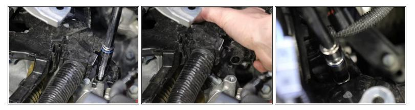
Unbolt the wiring harness and move it out of the way, exposing the shifter cables and bracket.
