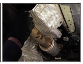
Remove the heat shield bolts and slide it out of the way, exposing the shifter cables.
