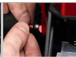
Attach the shifter cable end links to the shifter.
