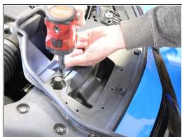
Begin in the engine bay by removing the air intake seal. You will need to remove the airbox lid so remove this section to make gaining access to the tray easier.
