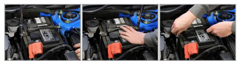
Remove the battery tie-down bracket.
