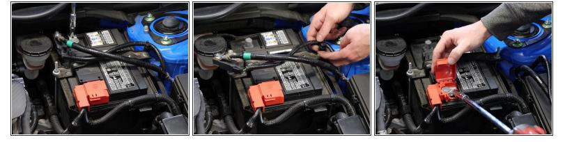
Remove the negative then positive terminal from the battery.
