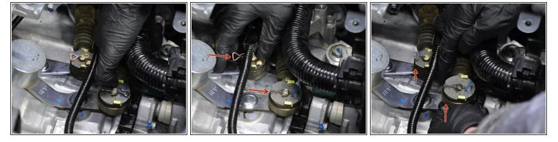
Remove the shifter cable retaining clips.
