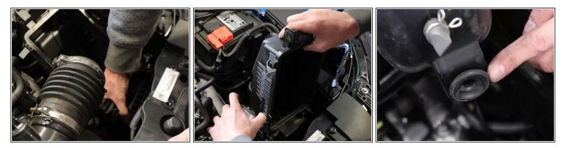
Grab the bottom airbox and pull upwards, the lower section is held in place by a grommet.
