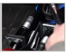
Now install the shifter cable retaining spring clips.
