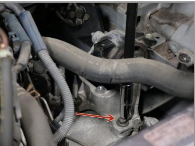
Remove the lower transmission bracket bolts.
