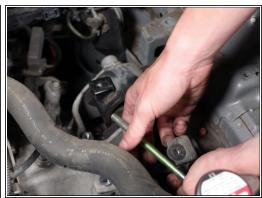
Remove the center bolt on the transmission mount.
