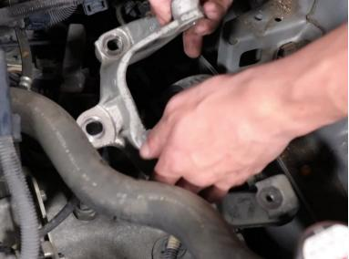
Remove the transmission bracket.
