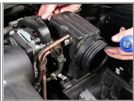
Remove the throttle body clamp.
