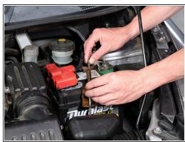
Begin by removing the battery bracket.
