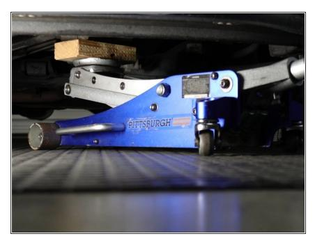
Locate a safe point under the transmission and use a floor jack to support the transmission while you remove the trans mount.
