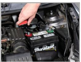
Remove both terminals and then remove the battery from the car. Set these parts to the side.
