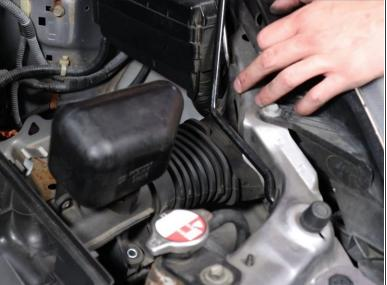
Remove the airbox tube and remove the airbox assembly.
