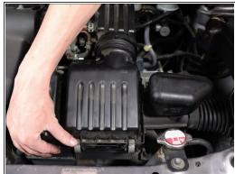
Unclip the four clips holding the airbox lid in place.
