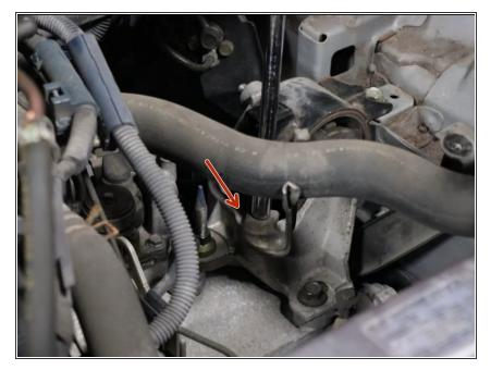
Remove the coolant hose bracket from the top of the transmission bracket.
