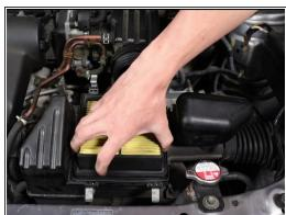
• Remove the air box lid and then remove the air filter.
