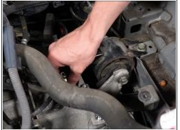
Remove the transmission bracket.
