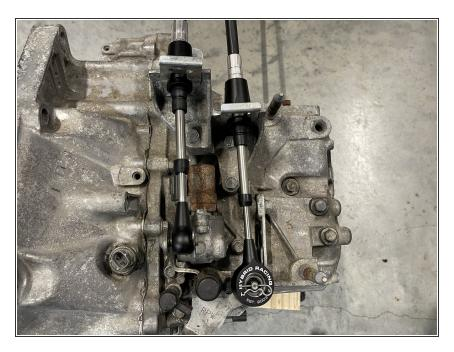
The cables should be completely connected to the transmission at this point.
