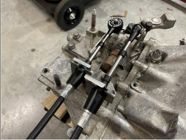
The cables are now installed. Depending on the application, be sure to keep the cables away from all heat sources.
