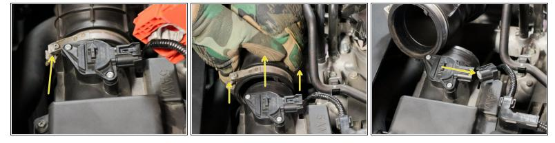
• Loosen the intake tube clamp, slide it off of the airbox and then unplug the MAF sensor.
