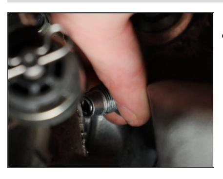
Remove the detent bolt and spring and set aside.
