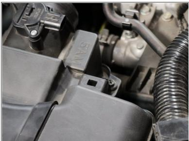
Remove the wire harness from the airbox.
