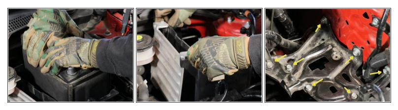
Remove the battery, heat shield and unbolt the lower battery tray.
