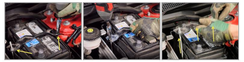
Unbolt the battery tie-down bracket and remove it.
