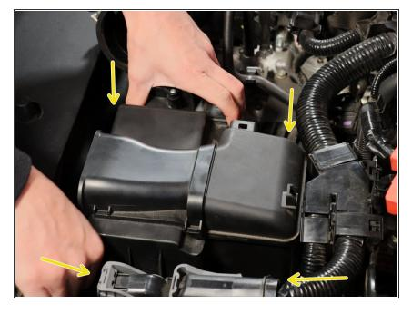
Unscrew the upper airbox lid. There are four screws that hold it in place.
