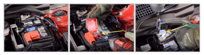
Begin by disconnecting the positive terminal battery, then remove the negative terminal.
