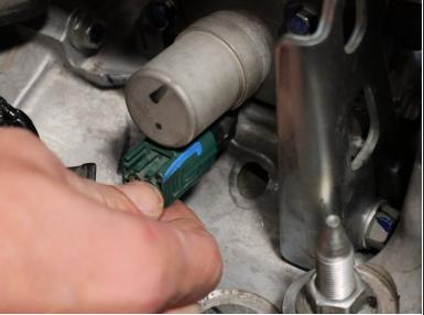
Locate the reverse solenoid on the top of the transmission and unplug the green connector.
