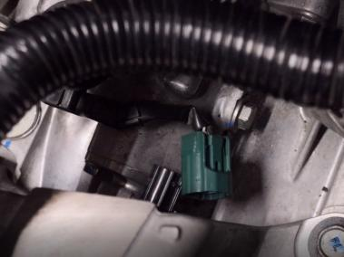
Unplug the reverse sensor on the top of the transmission.
