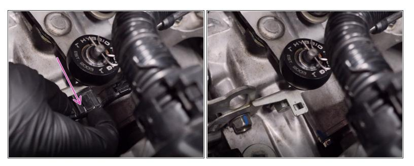
Remove the wire harness from the bracket on the front of the transmission.
