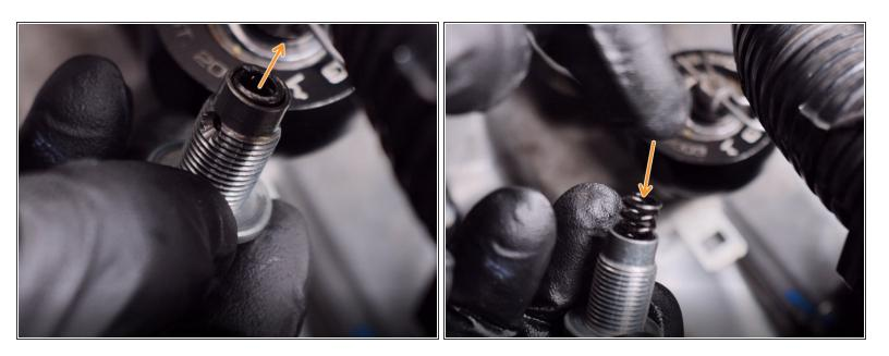
Install the new HR detent spring and re-install into the transmission.
