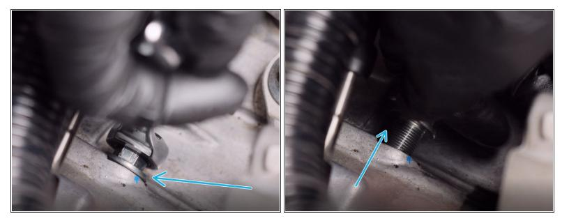
Locate the side detent spring and remove it.
