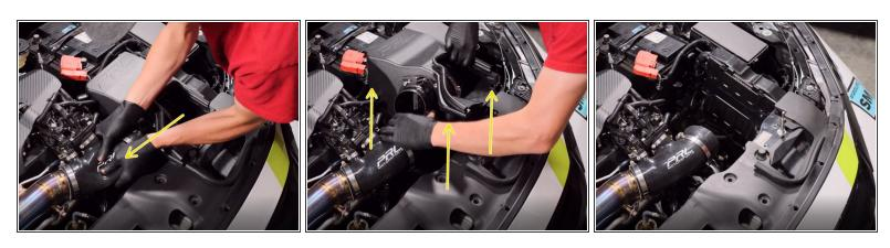
Pull the coupler off and remove the airbox from the car.
