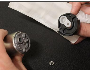
Use a flat-tipped screw driver or pry tool and remove the metal retaining clip holding the pick-up filter in place.
