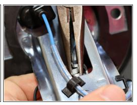
Install the rubber hose on the new Hybrid Racing fuel pump. Be sure to use the included line and clamps if your hose is not in good shape.
