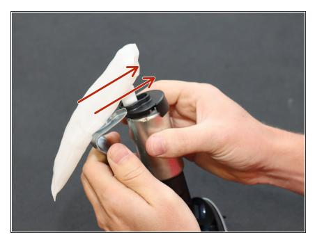
Remove the lower section of the fuel pump by sliding the rubber bushing out of the holder.
