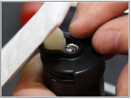
Install the OEM rubber bushing on the new Hybrid Racing fuel pump. Use the supplied pick-up filter and retaining ring as well.
