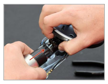
Disconnect the fuel pump by depressing the wire harness connector and pulling it outward.
