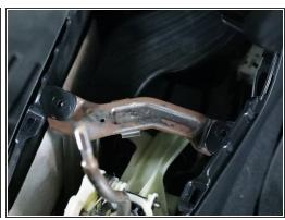
Use a Phillips screwdriver and remove the two screws that hold the console bracket in place.
