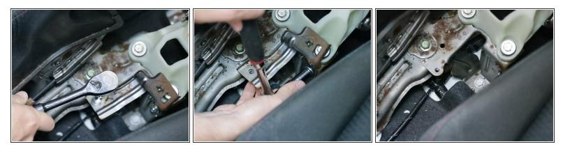
• Use a 10m socket and remove the steel bracket located behind the shifter.
