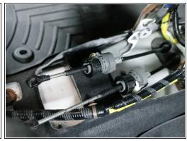
• Use a 12mm socket and remove all four bolts that hold the shifter in place. Remove the shifter from the car.
