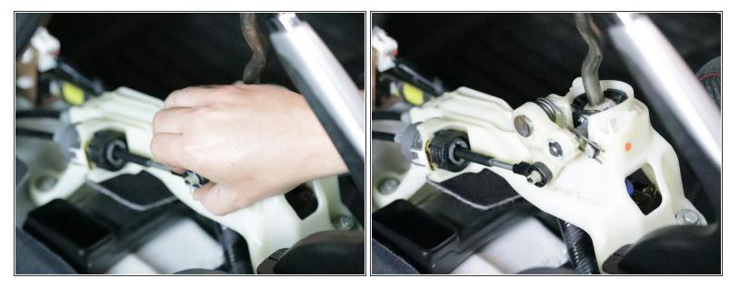
Remove the left side shifter cable by removing the retaining pin.
