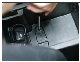
Inside of the center console armrest, there are two screws located under the felt liner. Remove them.
