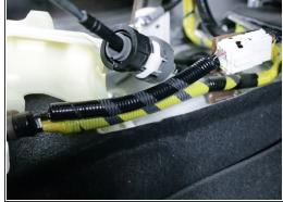
Repeat step 13 on the right-side cable. Spin the lock, slide it out and let it spin back once it is off the shifter. Keep this in mind as you will need to use the same technique to install them onto the new shifter.
