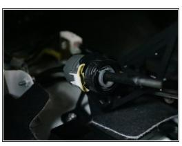
Refer to step 13 & 14 and re-install the shifter cables onto the Hybrid Racing shifter.
