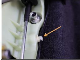
• Use a plastic pry tool and remove all (x5) plastic wire harness clips from the OEM shifter.
