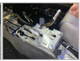
Lift the console from the rear and slide it rearward. Lift it over the shifter and remove it from the car.
