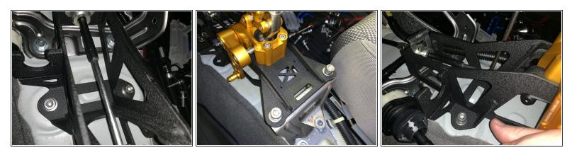
Install the Hybrid Racing shifter and use the supplied bolts to mount it directly to the chassis. It does not use any sort of base bushing.
