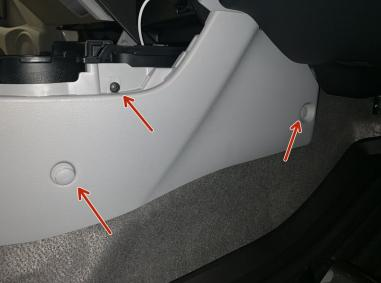
Remove the console clips and screws. There are two clips and one screw on each side.
