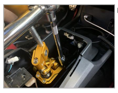
If you chose to change the inner spring, use a torque wrench and tighten the bolts to 6ftlb / 72inlb.
