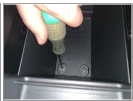
Remove the two screws inside of the center console.
