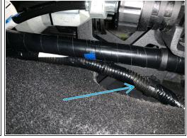
Reinstall the factory wiring harness onto the base of the Hybrid Racing shifter.
