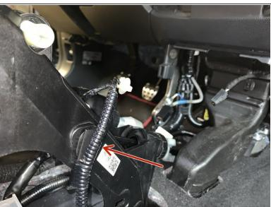
Remove the clips that hold the wiring harness to the factory shifter.
