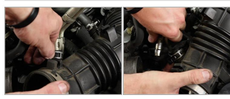
Unclamp and remove the valve cover vent tube from the intake tube.
