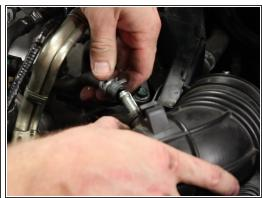
Unclamp and remove the air assist valve tube from the intake tube.
