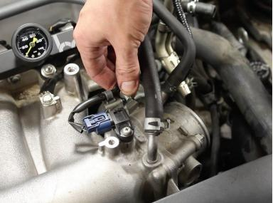
Remove the 10mm bolt mounting the MAP sensor harness mounting bracket.
