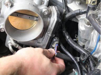
Plug in the throttle body harness to the new throttle body.
