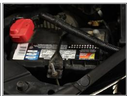
Using a 10mm wrench, disconnect the negative battery terminal.
