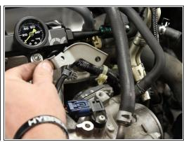
Unclamp the MAP sensor wire harness from the bracket and discard the bracket.
