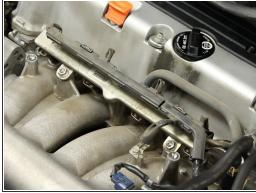
Remove the upper engine cover mounting studs. (3)
