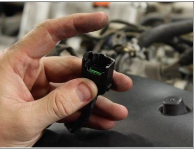
Using a small flat tip screw driver or pick tool, remove the pin lock inside of the OEM fuel injector connectors. (qty 4)
