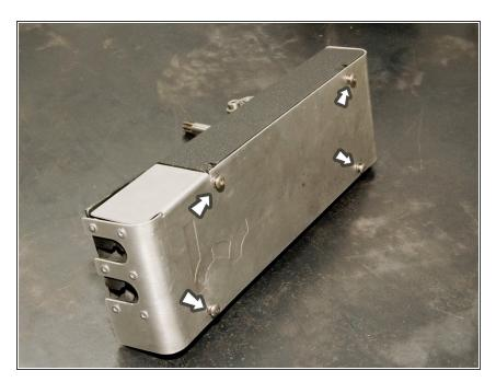
Using a 3mm allen wrench, unscrew the four M5 dust cover bolts.
