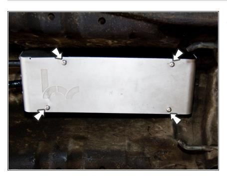
Bolt the debris shield that you removed earlier back onto the shifter.
